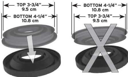
**NOTE:** There is a top and bottom to the gasket. The top measures 3-3/4 inches and the bottom measures 4-1/4 inches. The gasket fits snugly in the bottom cap.
