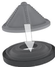
3. Screw bottom cap into the chute and blade cover.
